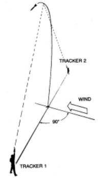
Each tracking station takes its own measurements of the angle reached. Both heights are calculated. The two results are averaged, and the average is used at the height reached. Usually both heights will be thrown out if they are not within ten percent of each other. This assumes that at least one of the tracking stations made a mistake and the results cannot be considered reliable.
