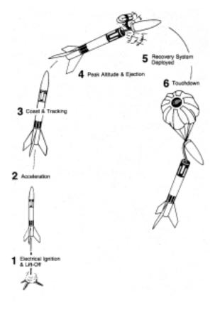
lasts until the engine has consumed all its propellant. During this phase, model rockets accelerate positively.
