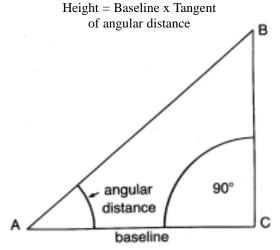
If we assume that the rocket flight is vertical, we can call angle C a right angle, 90 degrees. B is equal to 90 degrees minus A, because the sum of the angles in a triangle is 180 degrees. To find the distance from C to B or the height the rocket
