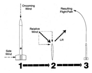
As you can see, the fin is the stabilizing and guiding unit of a model rocket. It should be in a symmetrical form of three, four or possibly more fins and made of reinforced paper, balsa or plastic. The fin is an aerodynamic surface projecting from the rocket body.
