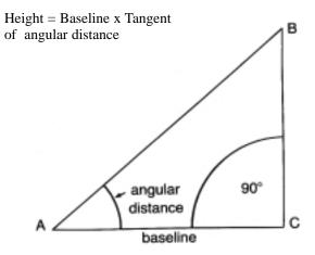
If we assume that the rocket flight is vertical, we can call angle C a right angle,  $90^{\circ}$ . B is equal to  $90^{\circ}$  minus A because the sum of the angles in a triangle is  $180^{\circ}$ . To find the distance from C to B or the height the rocket reached, take the tangent of Angle A times the distance along the baseline, side AC.
