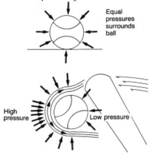
Pressure drag is the retarding force caused by the imbalance of air pressures on a moving abject. Pressures on a moving object vary with the object's speed, direction of motion and its size and shape.
