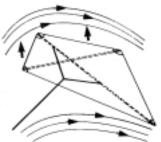
Lift is generated by *relative wind*. Relative wind is the motion in air in relation to an object, such as a kite in a breeze. It can also be created by running with a kite, if no wind is blowing.
