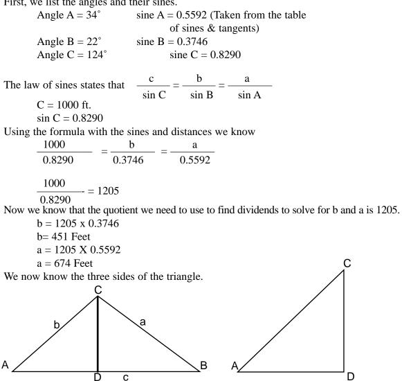
The altitude of the rocket is the distance from D to C in the diagram. The angle formed by the meeting of AB and CD is a right angle. The sine of an angle in a right triangle is the relation of the opposite side to the hypotenuse. We want to determine the value of the opposite, CD.
