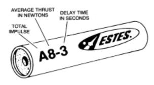
The engine code on each engine consists of a letter, a number and another number preceded by a dash. The letter indicates the average thrust of the engine. This value is in newtons . The last number is the delay time in seconds between the time of the engine's burnout and the activation of the ejection charge.
