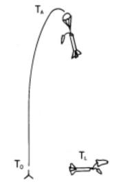
On the diagram, distance traveled is the distance between  $T_0$  and  $T_A$  (launch to apogee). That is the altitude or height the rocket reached at apogee.
