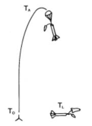
On the diagram, distance traveled is the distance between  $T_0$  and  $T_A$  (launch to apogee). That is the altitude or height the rocket reached at apogee. Use the following example data:  $T_0 = 0$  seconds
