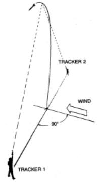
The two results are averaged, and the average is used as the height reached. Usually both heights will be thrown out if they are not within ten percent of each other. This assumes that at least one of the tracking stations made a mistake and the results cannot be considered reliable.
