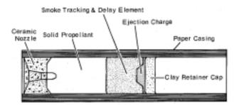
Model rocket engines are manufactured in a range of sizes. They come in over thirty varieties, each one varying in total impulse, average thrust, thrusting time and time of delay between propellant burnout and activation of the ejection charge.
