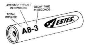
The engine code on each engine consists of a letter, a number and another number preceded by a dash. The letter indicates the total impulse or power of the engine. The number indicates the average thrust of the engine. This value is in newtons. The last number is the delay time in seconds between the time of the engine's burnout and the activation of the ejection charge
